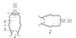
Material: Spring Steel Finish: nVent CADDY Armour
